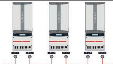
Wiring via RJ45 connectors
